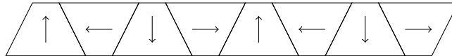
FIGURE 1.12: A segmented linear Halbach array made using trapezoidal prismatic magnets. These are able to achieve a stronger field than traditional cuboidal Halbach arrays [44, 48].
